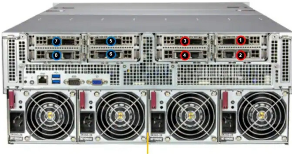
4 Redundant 3000W Titanium Level Power Supplies
